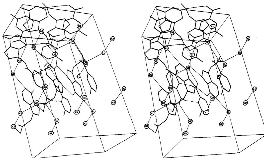
Figure 4. A stereoscopic view of a portion of the crystal structure illustrating the packing relationships among its molecules. Covalent bonds are shown as thick lines, unit cell outlines and hydrogen bonds are shown as thin lines and C-H...O hydrogen-bond-like interactions are shown as dashed lines. Water oxygen atoms are represented as thermal ellipsoids such that the vibrating atoms have a 25% probability of being found within them. Hydrogen atoms have been omitted for the sake of clarity.
